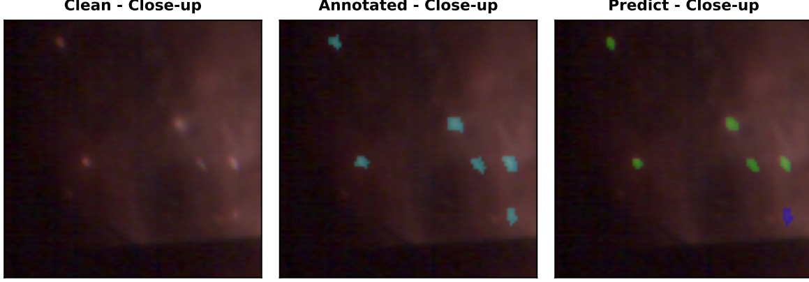
Fig. 5 Segmentation close-up from Fig. 3. Left: raw image. Middle: ground truth annotation. Right: model segmentation output (green denotes true positives and blue denotes false negatives).
